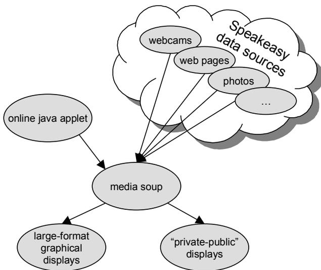
Figure 3: Users can add content to the soup by connecting Speakeasy sources to it or via the online Java applet. Data is extracted from the soup for viewing on public or private-public displays.
